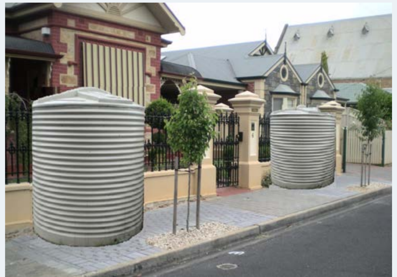
Above image: The rainwater tanks represent the annual amount of water (4000 litres) delivered to the soil through 8m 2 of permeable pavement. Photograph taken 29 October 2010 (Johnson, 2022).
